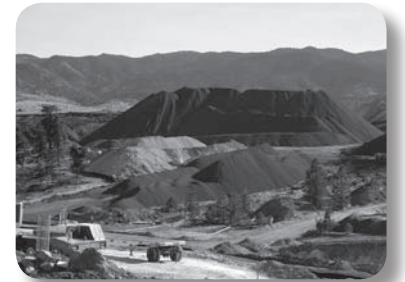
Mountain of concrete aggregates (gravel) being manufactured by Fisher Industries to make concrete for the I-580 project.
